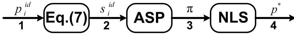
Figure 2 Follower system: receives a desired bit-map p and returns a feasible bit-map p^* , with the nearest result to the input
